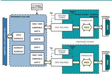
PCI Express Mini Card (mPCIe), a low-profile small-footprint bus standard originally intended for adding peripherals to notebook computers, has become the de-facto standard for highperformance, small form-factor devices in many applications.
